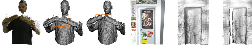
Fig. 12: Effect of connectivity update. Left: input point cloud. Middle: result without connectivity update. Right: result with connectivity update.
