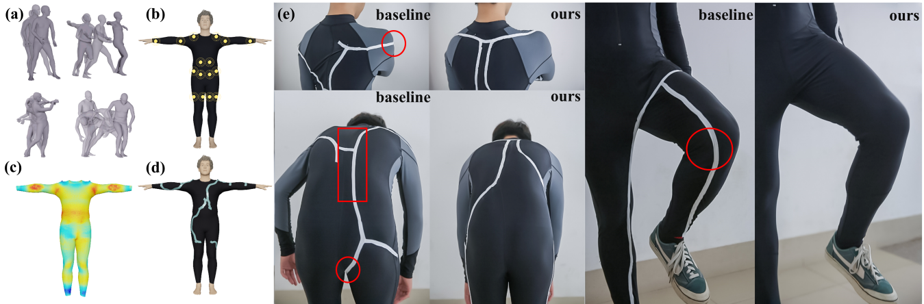
Fig. 1. Designing wiring layout on tight suits. Given a set of motion data (a) and on-garment terminals (b), the goal is to find the wire layout connecting the terminals, while minimizing motion resistance when the user is wearing the tight suit. We analyze the cloth strain deformation (c), and obtain the wiring layout (d) by resolving a deformation-weighted Steiner tree problem. User experiments show that our approach can effectively reduce the deformation strain at various body parts (highlighted in red boxes) compared with a minimum-length baseline approach (e).
