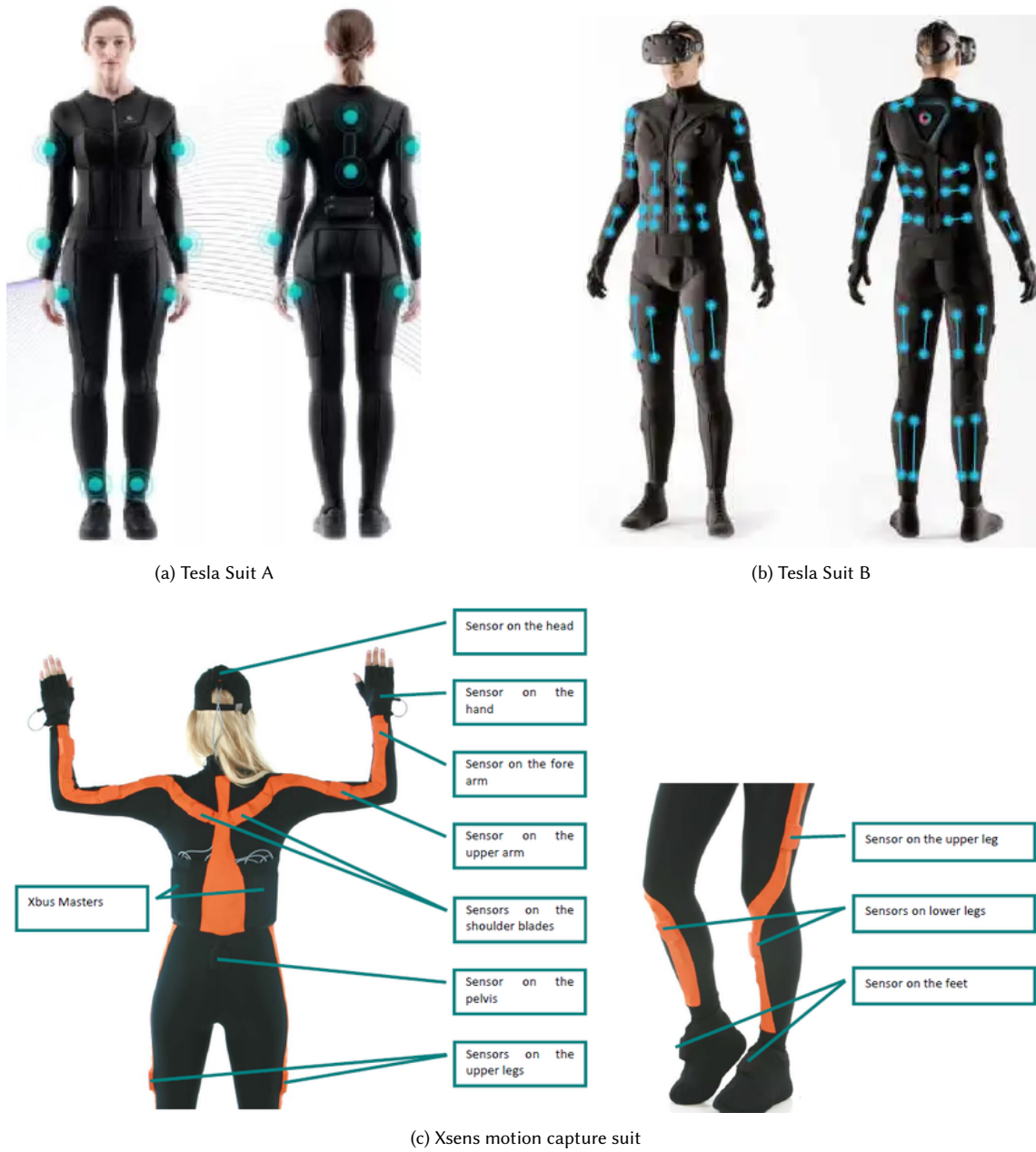
Fig. 7. Three commercial products of smart clothing used in our work for layout reference design.
