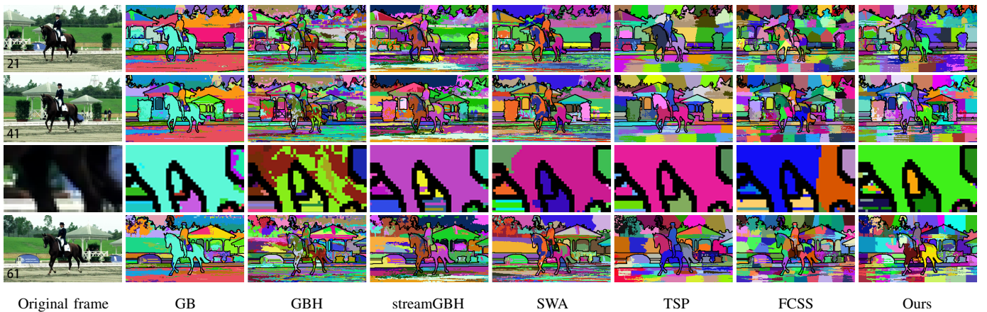
Fig. 1: Segmentation results of representative algorithms, such as GB [16], GBH [20], streamGBH [43], SWA [35], [36], [10], TSP [8], FCSS [46] and ours. The magnified details in the third row show that our method is sensitive to color changes and achieves better boundary adherence. For 500 supervoxels, our processing speed is at least 20 times faster than FCSS and 100 times faster than TSP. See Section V for detailed comparison results.
