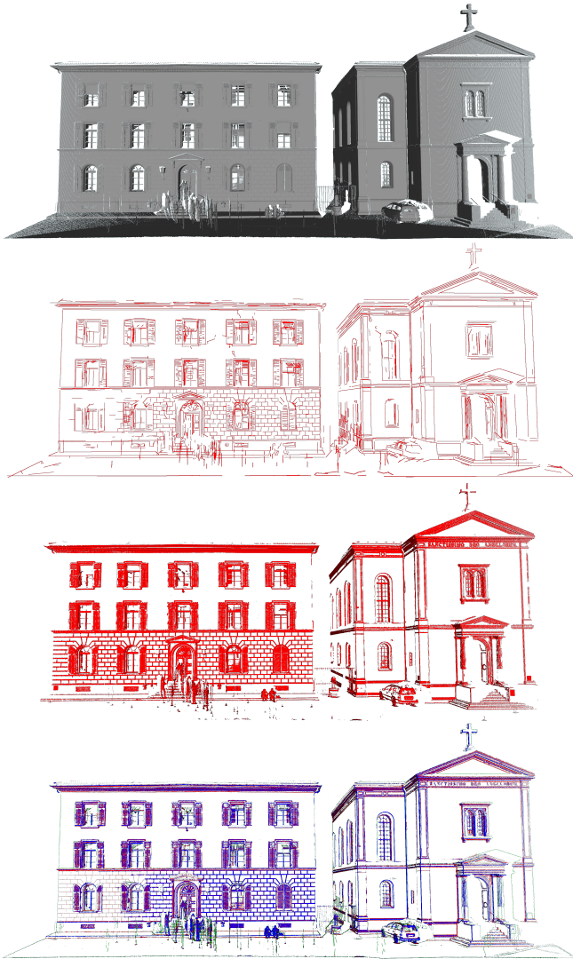
Fig. 9. Comparison experiment between F3D [42], PCA [32], and NRLC on the second LiDAR building point cloud. From top to bottom, these figures are the input model, feature sets generated by F3D, PCA and NRLC.
