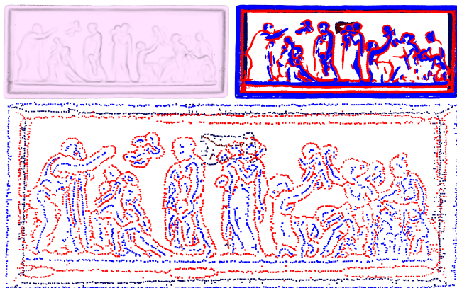
Fig. 4. NRLC produces geometric features (top-right) for a relief point cloud (top-left). The thin relief features (bottom) are generated by first implementing a set of assimilations and then enforcing another set of dissimilation operations on the thick feature sets.
